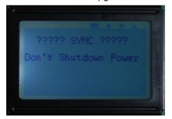
7. Run updater V1.2.exe on your computer upgrade software, if the upgrading software normal operation, it will appear the interface as follows
