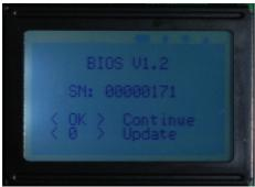
6. Input 0 in keyboard, when appear the following interface, it means the device has entered the state to upgrade.
