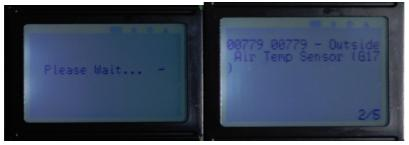
Note: Press <↓> keys to read the next fault code, and <↑> key to read the last fault code, press BACK button to return to previous menu. Fault code also supports multi-language
