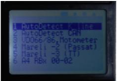
b) According to the type of odometer, select the corresponding option. Maily odometer is divided into K line and CAN line, but the K line and CAN have different manufacturers, different versions, different types of odometer. User can choose K-line or CAN line automatic way, for some special odometer, user have to select the corresponding instrument through the menu. After choosing, press OK key, appear the following information:
